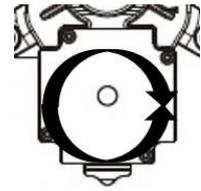
The motor arm must reach and touch the corresponding limit screw in order for the barrier to lock into terminal position.
